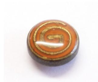
A clear epoxy added over the face of the rivet.
